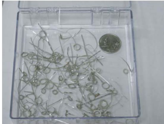
Figure 3.6: A mass grave of millitrap coils which did not survive the construction process. A U.S. quarter is included for size reference.
