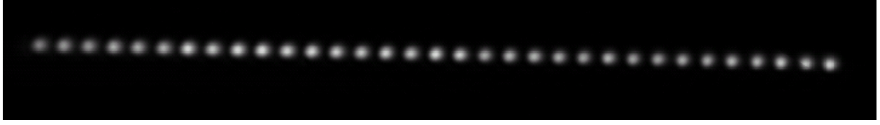
Figure 7.2: (33x) focused laser spots generated by imaging the AOD output using the high-NA objective. Here we see some variation in the intensity of the the different tweezer spots. In an experiment this intensity variation would need to be calibrated out and compensated for.
