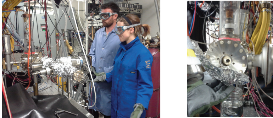
Figure 3.3: These pictures are from the oven change of 2013. On the left, Thomas Barter and I prepare to open the right angle valve that separates the RGA and turbo pump from the oven chamber. While flowing gaseous nitrogen through the chamber, we remove the oven from the chamber. The copper cold catcher is visible through the opening. It is covered in rubidium so that it appears white. We clean the rubidium off of the cold catcher before replacing the rubidium ampule.
